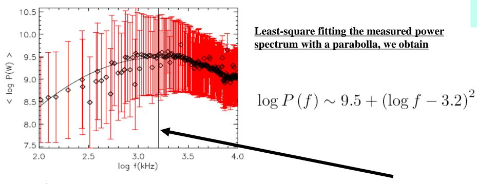
The spectrum presents a maximum of emissivity around 3 GW at 1.5 MHz
